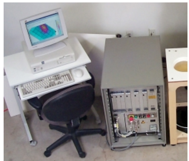
System Controller with Application Software, robot controller.
