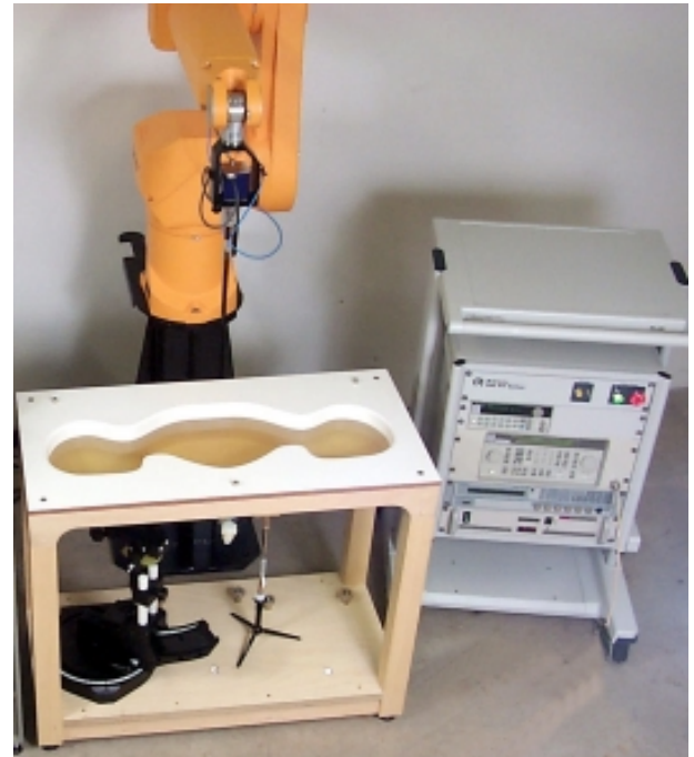
SAR System Components – robot with probe, twin phantom and integrated table, validation instrumentation in mini-rack, dipole antenna, and EUT mounting device.
