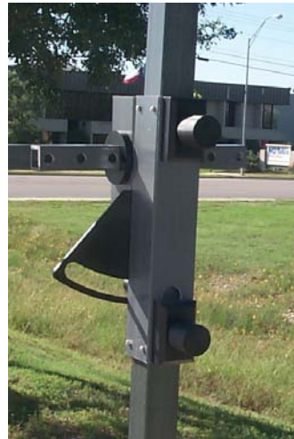
2. The positioning gimbal secures the mounting arm to the mast.
