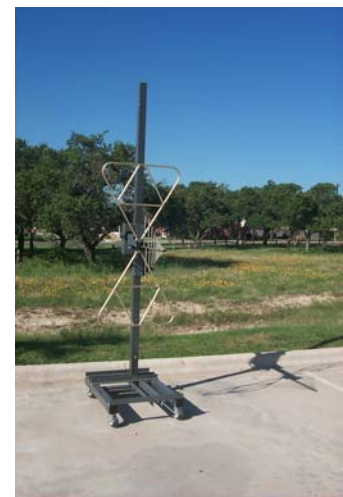
6. Antenna mounted on mast in vertical polarization.
