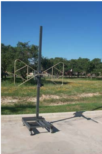
1. Antenna mounted on mast in horizontal polarization.
