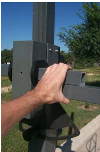
4. Manually rotate mounting arm 90 degrees counterclockwise.
