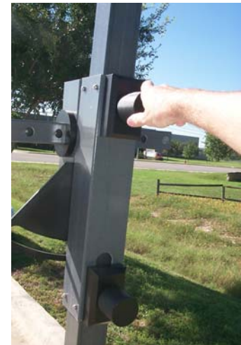
3. Place the stepladder next to the mast. Loosen the top vertical positioning screw.
